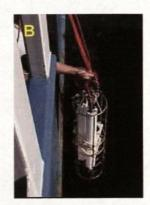
**Figure 5. 4** VIP systems in titanium frames were deployed simultaneously (B) with 2 VIPs in one frame (A1), 2 VIPs and an ocean 7 CTD probe (A2) and MPCP (A3).
