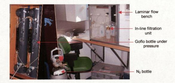
Figure 5. 7 The filtration set-up. Go-Flos were pressurised and connected to an inline filtration unit that was housed in a laminar flow cabinet.
