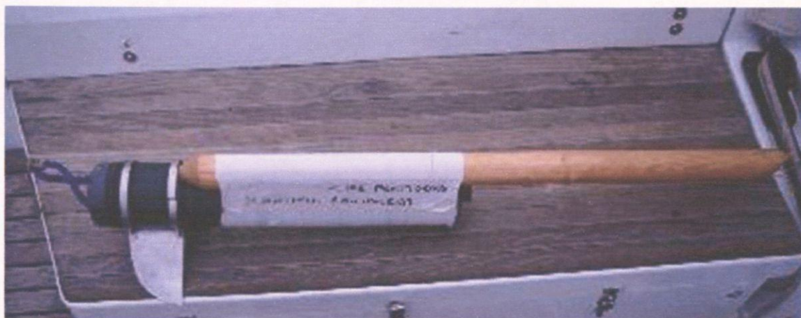
Figure 2: 2002 T-POD showing the buoyancy tube and diving fins as fitted to the outer casing.
