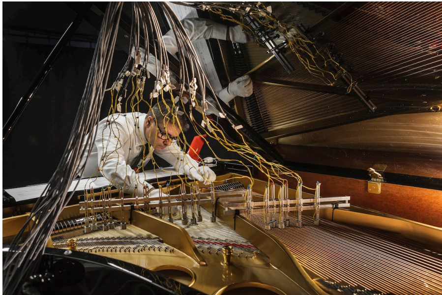
Figure 30: The biocomputer plays the piano through electromagnets placed close to the strings.
