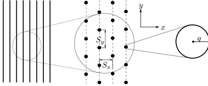
Figure 1: Schematic depiction of the array: Line array in the macroscale (left), individual absorbers in each line (center), and a single absorber of typical size parameter  $q$  (right).  $S_x$  and  $S_y$  are the device spacings in  $x$  and  $y$  directions, respectively.
