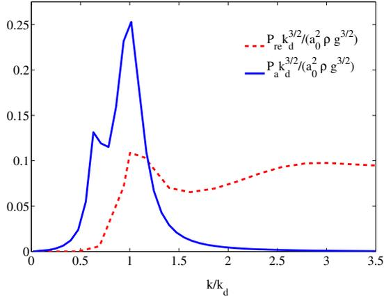
Figure 5: The dimensionless absorbed power  $P_a k_d^{3/2}/(a_0^2 \rho g^{3/2})$  (blue, solid line) and dimensionless reflected power  $P_{re} k_d^{3/2}/(a_0^2 \rho g^{3/2})$  (red, dashed line) for a twin cylinder WEC in heave, sway and roll with size  $qk_d = 0.65$  and damping coefficients  $C$  chosen for optimal power absorption in heave.
