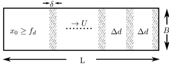
Figure 7: Schematic geometry of an ocean basin of length  $L$  with a number of wave-farms (shaded areas) a distance  $\Delta d$  apart. A constant wind  $U$  blows from the left, and  $x_0$  indicates the leading fetch prior to the first device, assumed greater than the fetch needed for a fully developed sea  $f_d$  under design conditions.  $\delta = S_x \cdot (N - 1)$  is the farm width, composed of  $N$  lines of absorbers, and  $B$  the harvesting breadth orthogonal to the wind direction.
