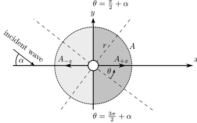
Figure 2: Schematic depicting the control surfaces  $A$  (dotted line),  $A_{+x}$  (right semicircle of  $A$ ), and  $A_{-x}$  (left semicircle of  $A$ ) at a distance  $r$  from the converter, used for the balance of power for a wave incident at an angle  $\alpha$  to the  $x$ -axis.
