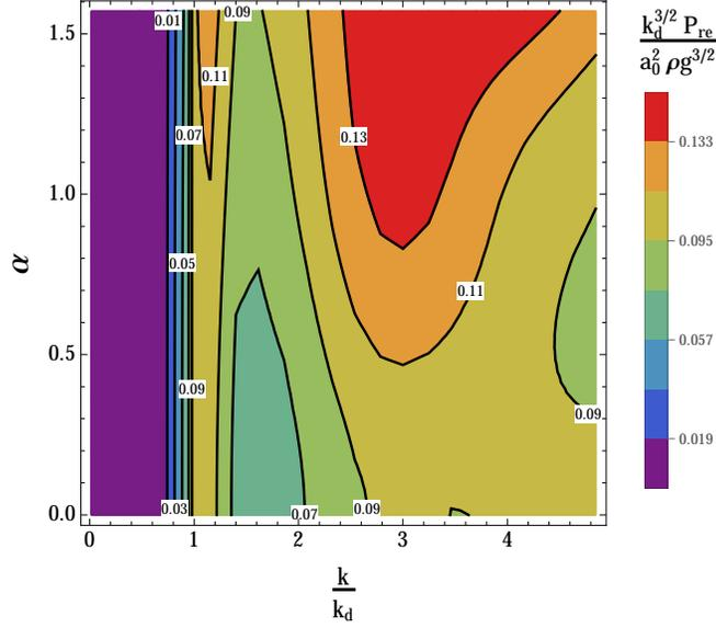
Figure 6: The dimensionless reflected power  $P_{re}k_d^{3/2}/(a_0^2\rho g^{3/2})$  of a twin-cylinder WEC attacked by a monochromatic wave with wavenumber  $k_d$  and amplitude  $a_0$  incident at an angle  $\alpha$ .  $\alpha \in [0, \pi/2]$  is plotted on the vertical axis.
