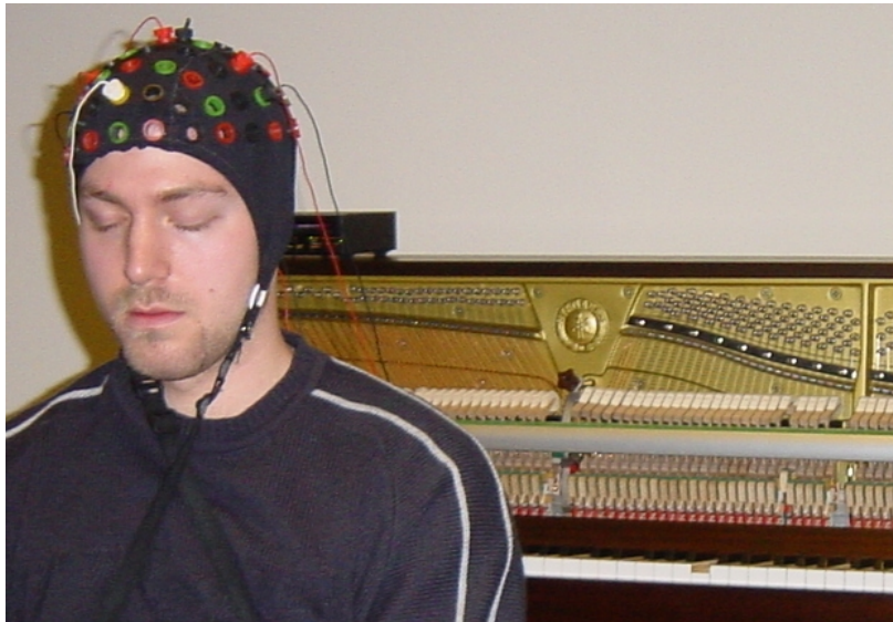
Figure 1.1: With BCMI-Piano one can play music generated on the fly on a MIDI-enabled acoustic piano with brain signals. No hands needed.
