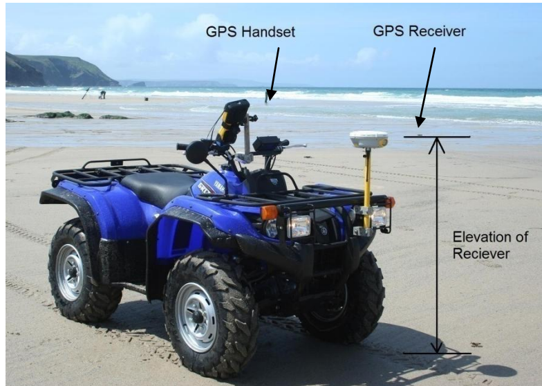
Figure 3.1–ATV with RTK GPS handset mounted on the handle bar and receiver mounted on the front luggage rack
