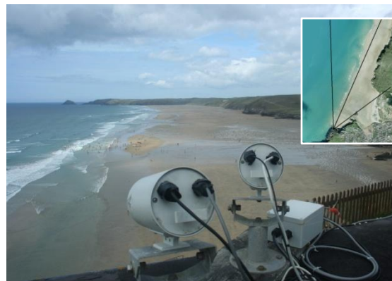
Figure 3.9– Argus cameras at PPT with the field of view shown on the aerial insert.
