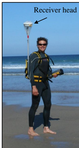
Figure 5.2– Photograph of the RTK GPS mounted on a surveyor for access to low tide regions during neap tide cycle during PX1, and for complete coverage during PX2.
