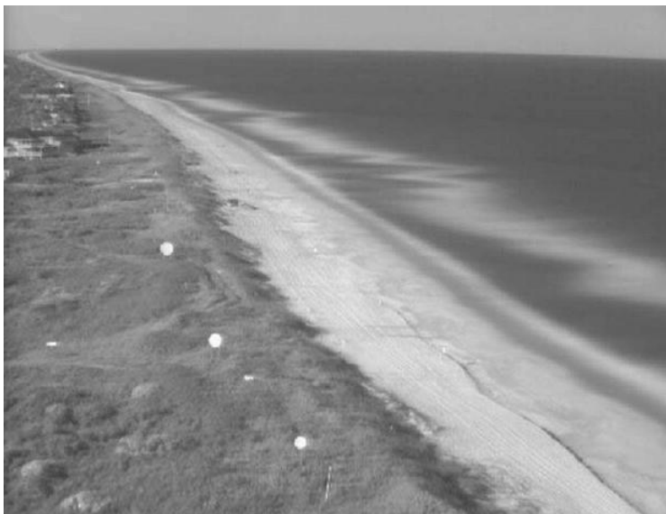
Figure 1.11 – Example Argus timex image showing bands of foam caused by wave breaking over a nearshore bar and at the shoreline, from Holman and Stanley (2007).
