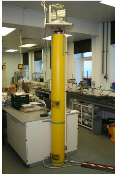
Figure 3.8– Settling tower used for sediment analysis. Scales are located at the top of the tower connected to a flat disc which is suspended 2.17 m below at the base of the tower.
