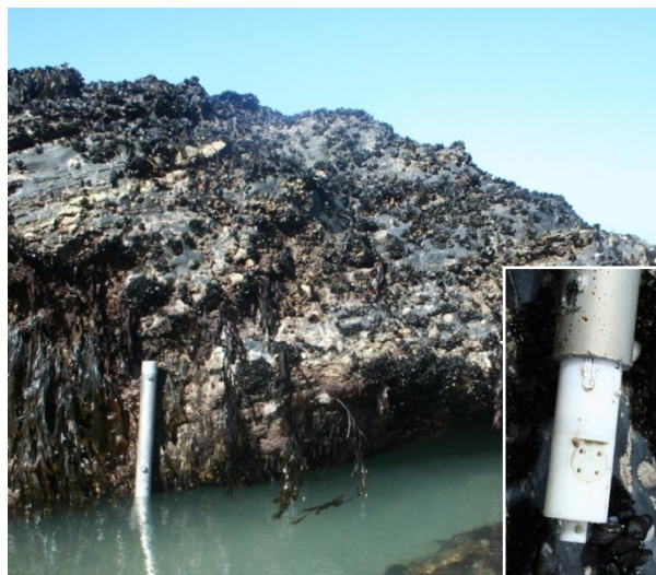
Figure 3.16–RBR TWR mounted to a low tide rock at PTN, insert shows the TWR extending from the scaffold tube during replacement.
