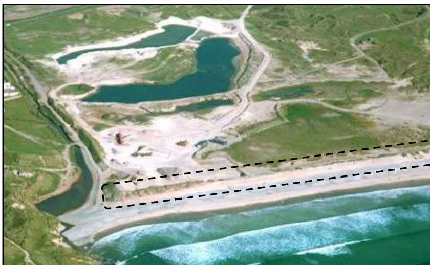
Figure 2.8 – Aerial image of previous sand extraction activities at Gwithian with the Red river to the left of the image. The artificial bund is highlighted within the dashed box.
