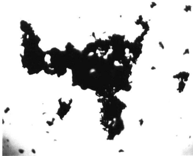
(ii) Ash from 1000 ^{\circ}\text{C} air burn off of \text{B}_2\text{O}_3 -doped coke.
