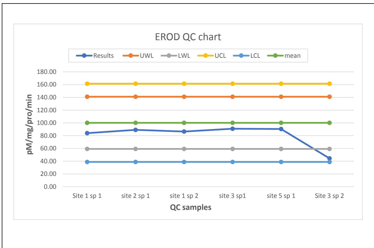
Figure 2.6 The control chart for EROD assay. None of the QC results were outside the deviation limits (UWL, UCL, LWL and LCL) except for the site 3 sp 2 sample that showed low EROD activity but still within the LCL. The QC samples were prepared by Cefas staff in 2010 in the Cefas laboratory at Lowestoft by measuring EROD activity in Dab ( Limanda limanda ).
