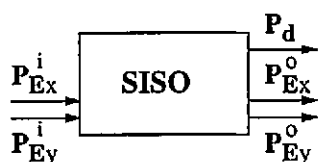
Figure 2.19: SISO decoder for the outer code
