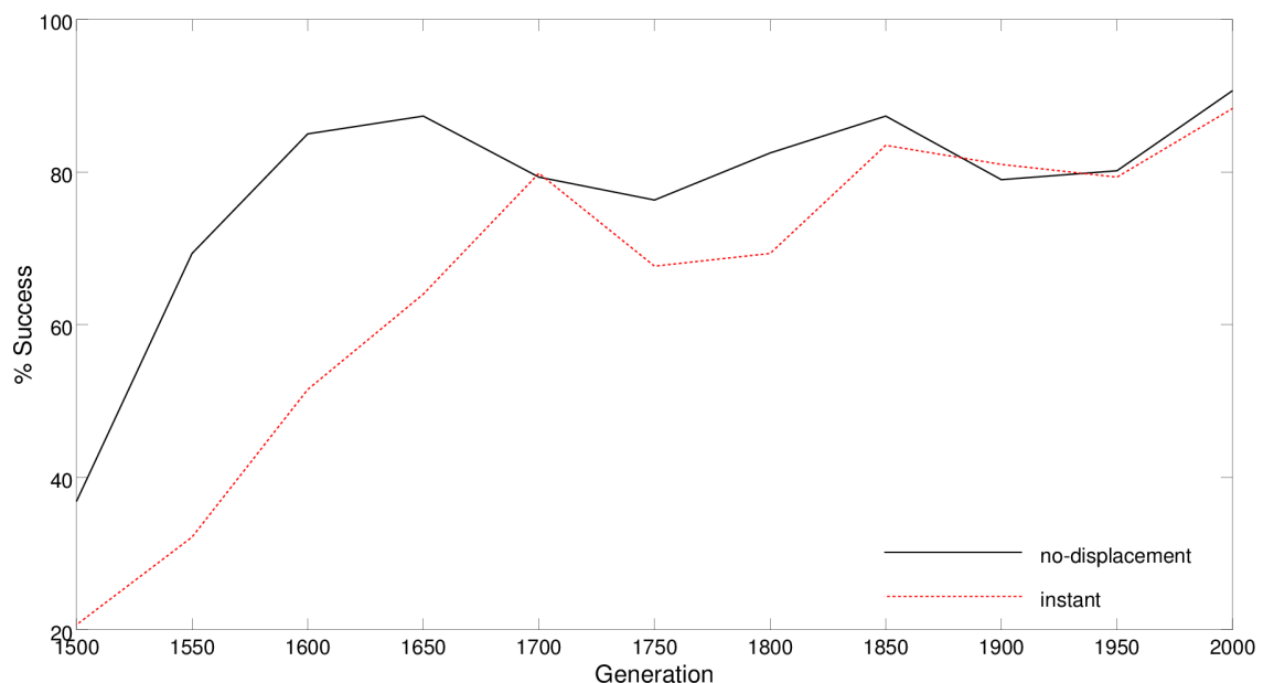
Fig 16. Performance displayed by the best CRp2 during the course of the evolutionary process in a no-displaced and displaced condition (black and red lines, respectively). In the latter condition the robot was allowed to move immediately after the displacement. Data were collected every 50 generations from generation 1500 to 2000 and averaged over 600 trials in the case of the no-displacement condition and 2400 trials in the case of the displaced condition. The displacement occurs when the robot reaches an imaginary line located 40cm before the first junction, or 40cm after the first junction, or in the middle of the horizontal corridor, or 40cm before the second junction.
