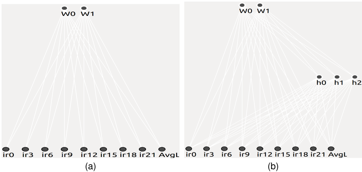
Figure 3.3: Range Neural Network Controller with (b) and without (a) hidden neurons. The output neurons W define the motor activation for left and right wheels of the robot. Neurons with a white contour around it mean the presence of a bias parameter. The input AvgL is the average activation of the rotating long range sensor.
