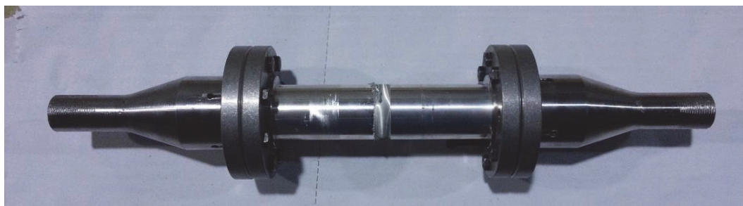
Figure 5: Complete assembled fatigue specimen and clamping fixtures.
