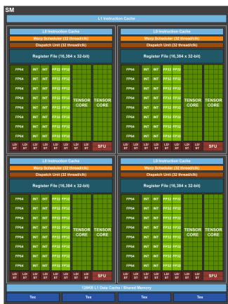
(a) GV100 structure.
