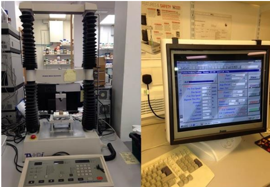
Figure 3.5: Texture analyser unit at Plymouth University
