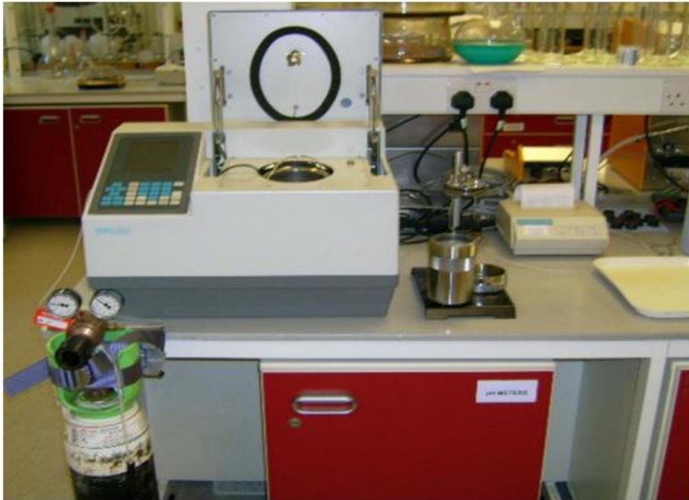
Figure 3.4: Bomb calorimeter at the nutrition lab at Plymouth University
