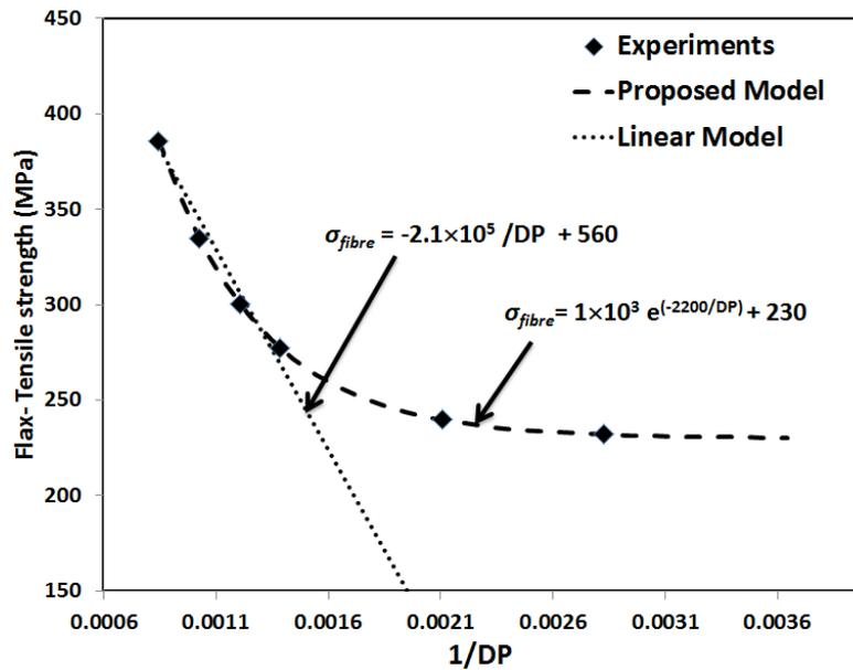
Fig. 5. Tensile strength vs  $1/DP$  for flax fibre at various temperatures and times.  $DP$  for flax was not measured but rather was calculated using data from Ref. [12] using Eqs. (3, 6, 11) and (15) with the measured temperature history.
