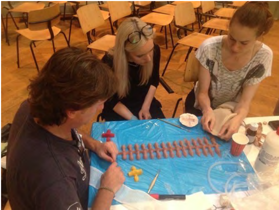
Figure 59. Agi Haines working with Ricardo Mutuberrria and Kim Jansen on the clay mould for a silicone casing inspired by the human spine.
