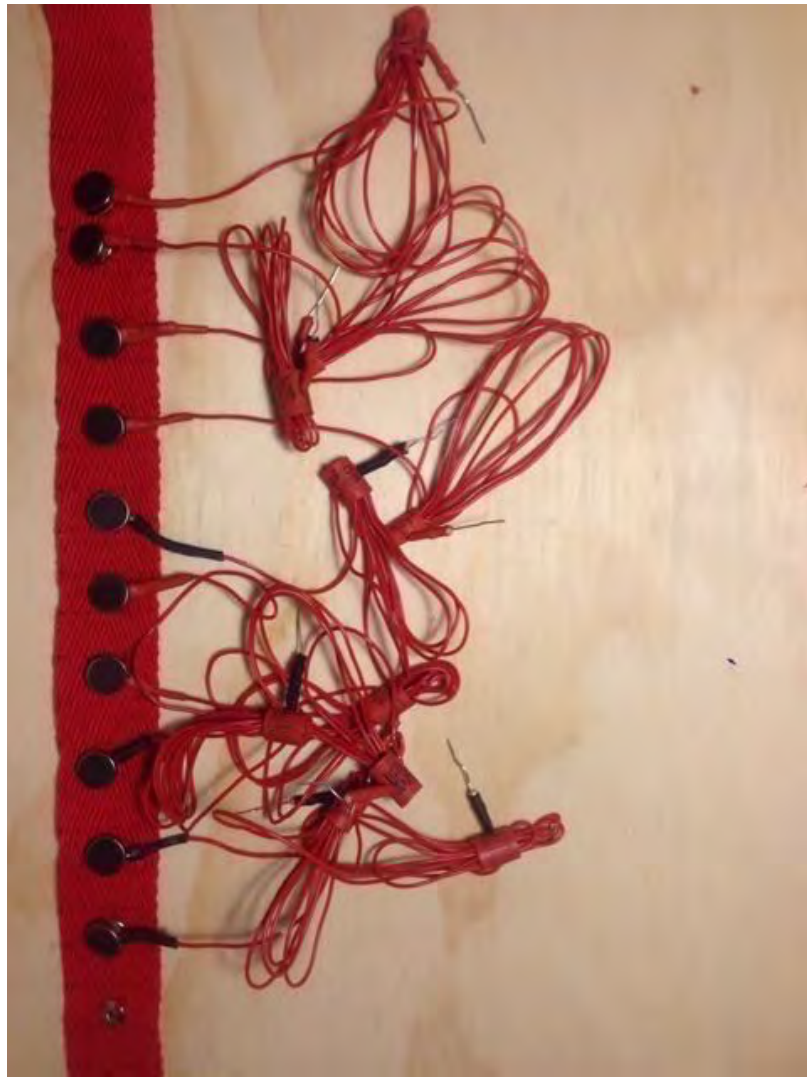
Figure 22: Early version of snaps sewn onto non-elastic fabric ribbon
