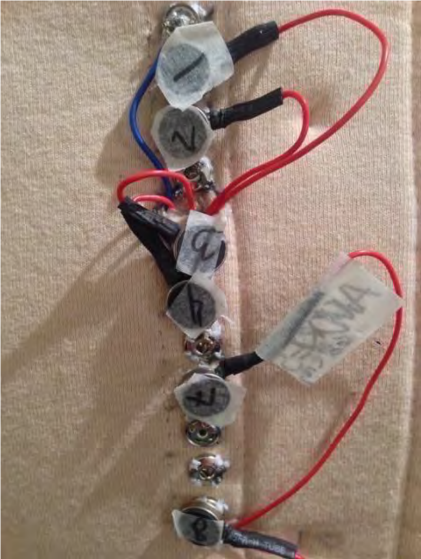
Figure 21: Conductive snaps were initially attached directly to the back support suit
