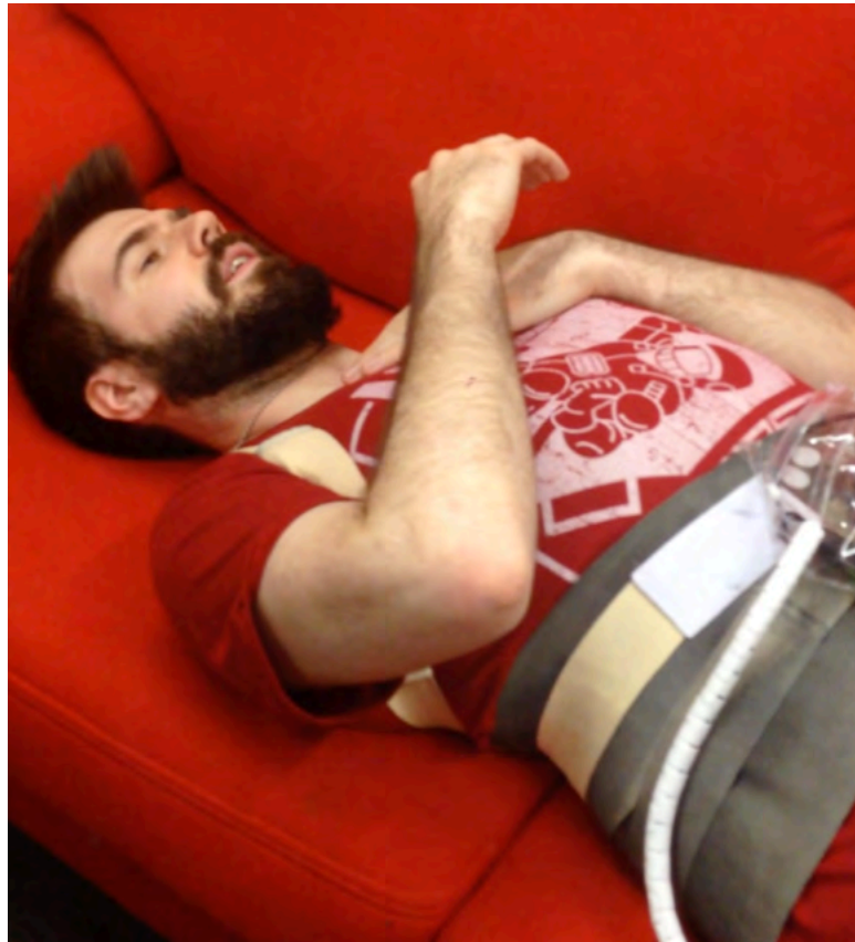
Figure 17. The motors are pressed against this participant's back as he lies prone on the couch, a position which also reduces postural tone.
