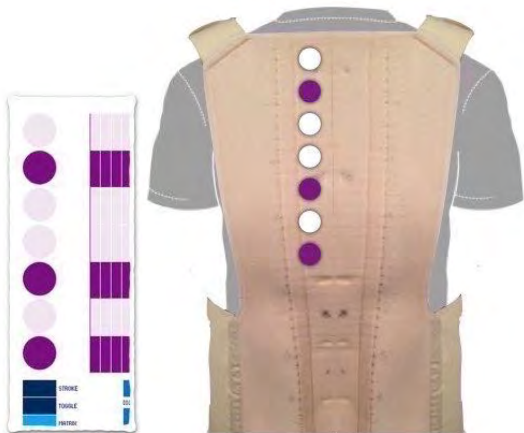
Figure 28: Visualisations of the motor activation shown on the GUI used in the Manufactory workshop and at the Bizarre Bazaar demonstration.
