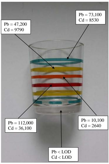
Figure 2: The distribution of Pb and Cd concentrations (in  $\mu g \, g^{-1}$ ) on the exterior of a lowball tumbler purchased from a supermarket. Note the deterioration of the lowest (blue) ring, evident at the time of purchase.
