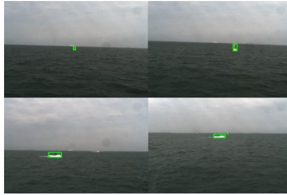
Figure 4. The obstacle is tracked among successive frames (Wang et al., 2011, 2012).
