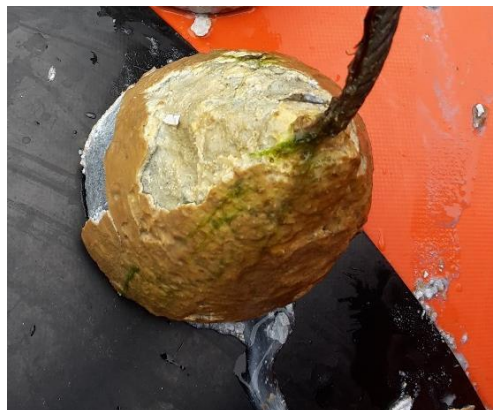
Fig 7 Anodes form a layer of zinc hydroxide and calcium if they dry out or are exposed to freshwater or brackish conditions, thus effecting corrosion rates
