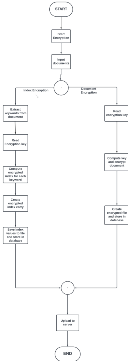
Figure 3: Flowchart explaining the index and document encryption process.
