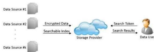
Figure 1: General SSE architecture where encrypted data is stored in the cloud and returns data when user queries after searching on encrypted data.
