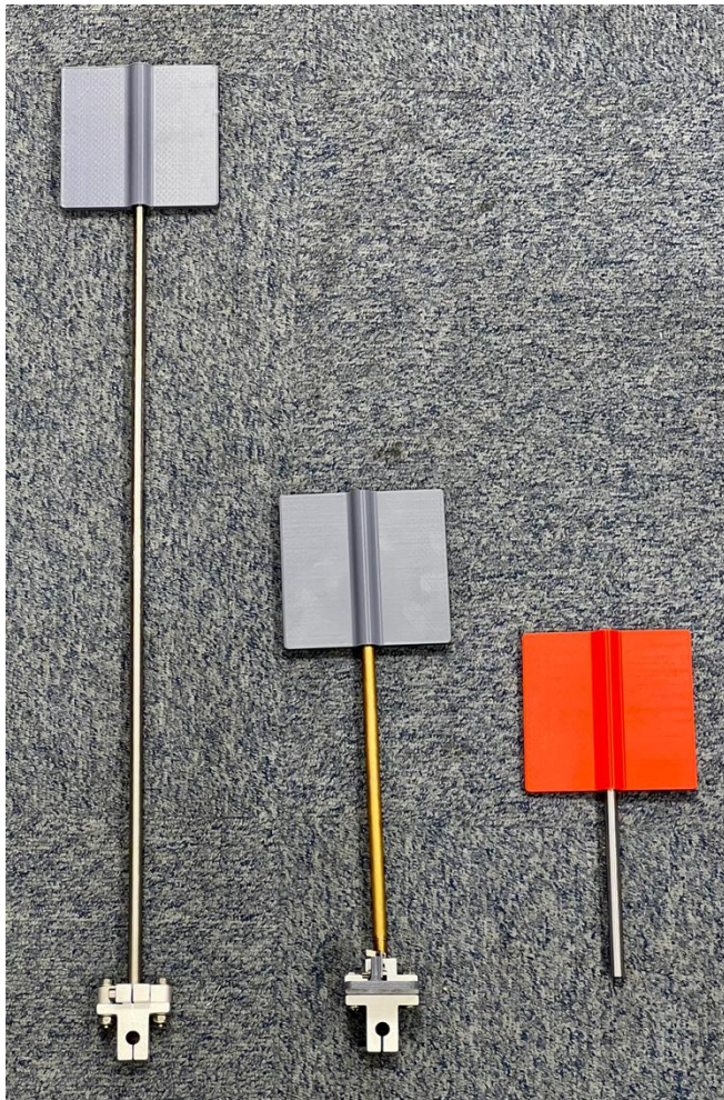
Figure 4: Three different pendulum poles were utilized to evaluate the controller's sensitivity to changes in pendulum length.
