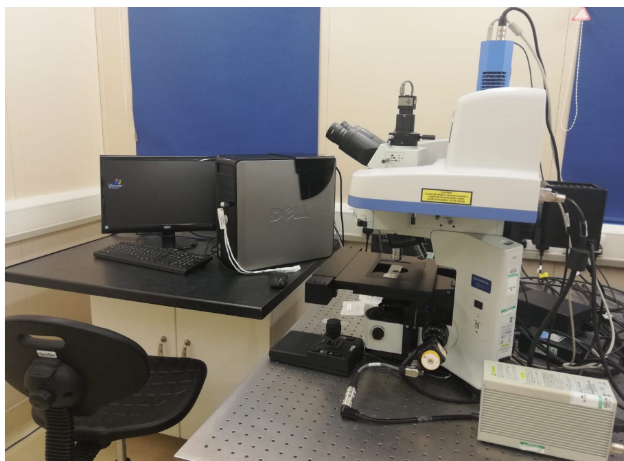
Figure 3.8: XPLORA HORIBA system combined with an Olympus BX41 microscope for Raman Spectroscopy
