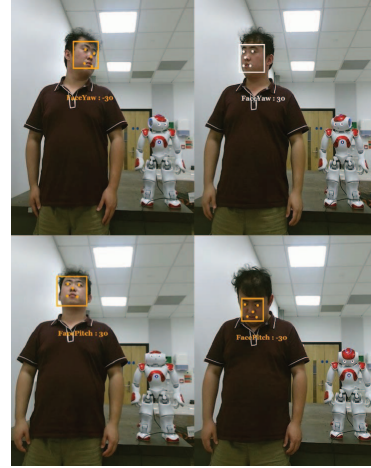
Fig. 10. Process of imitation for Nao robot head following: Rotating 30° to left and right directions and pitching up and down with 30°
