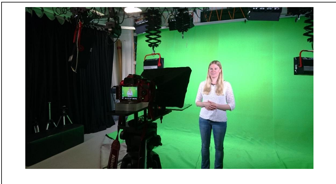
Figure 2.13. Studio recording of the reduced FIT script for the holographic projection using a teleprompter and green screen technique.
