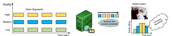
Fig. 9: Dynamic adaptation according to network conditions.
