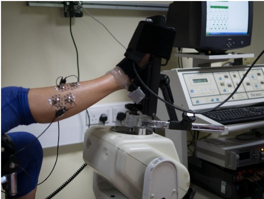
Figure 2.13 Position of participant in Biodex™ dynamometer for measuring ankle invertor stiffness
