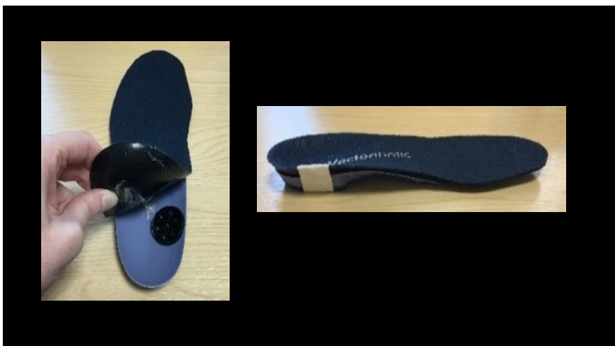
Figure 7.2 Positioning and blinding of the discs on the Vectorthotic™ shell
