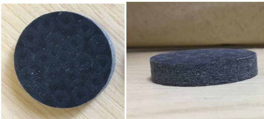
Figure 6.6 Second prototype of the cones orthotic component without open lumens in the cones
