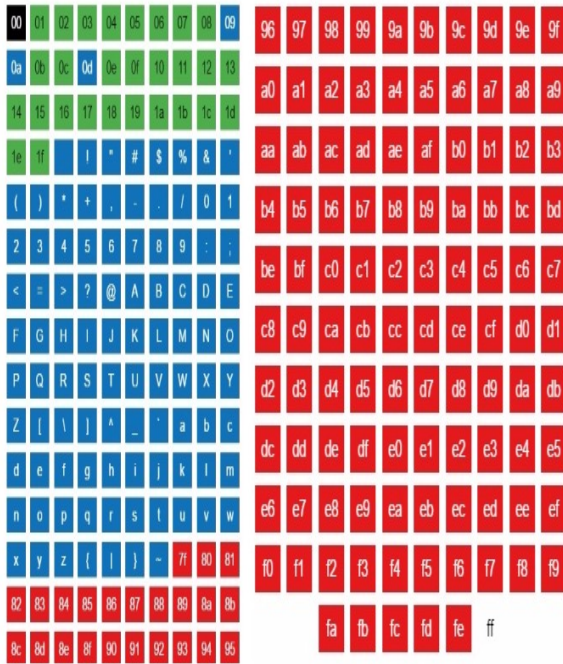
Figure 3: Binvis.io colour scheme. Tab (09), newline (0a) and carriage return (0d) are considered to be text (Cortesi, 2016).
