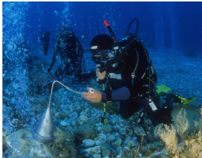
Fig.2. Venting gases sampled off the island of Panarea. The pyrex bottle was filled by sea-water before diving. The gas coming from the inverted funnel displaced the water allowing the collection of a gas sample without atmospheric contamination and with a pressure equilibrated at the sampling depth (overpressure).
