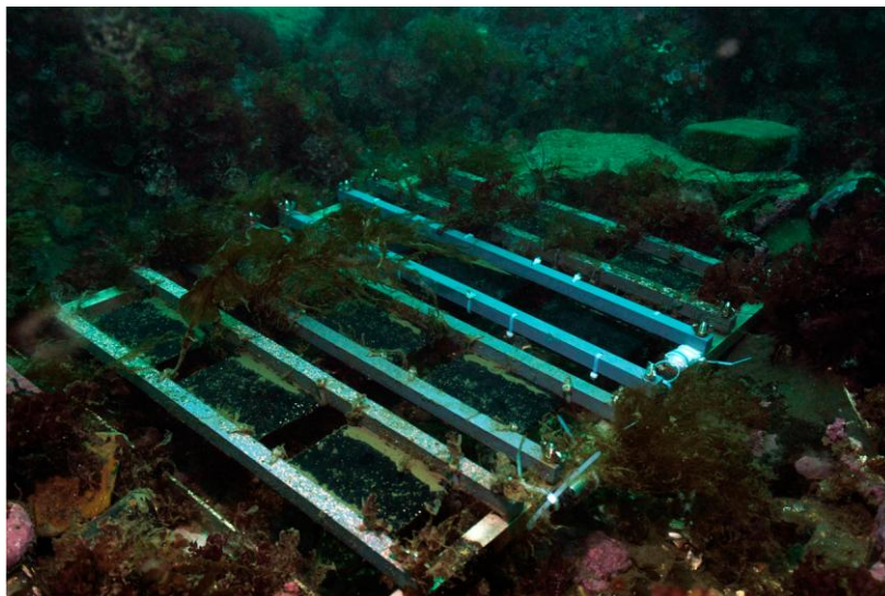
Fig.4. Hard bottom Arctic cryptic biota development project. Metal frame on which plastic panels are mounted mimicking hard substrate. Number of environmental data loggers attached to the construction.
