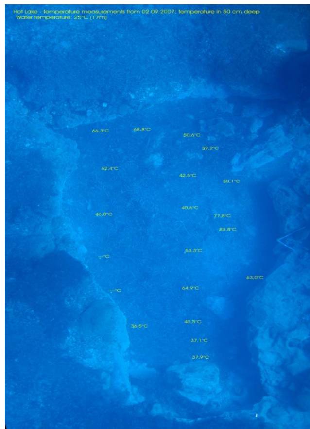
Fig.5. Temperature measurements in a depth of 50 cm at Hot Lake.
