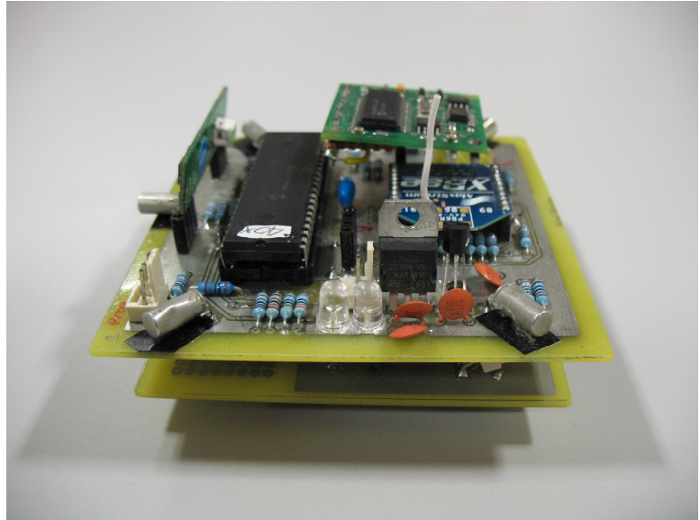
(fig. 33 Stacked PCB prototype with sensor integration)
