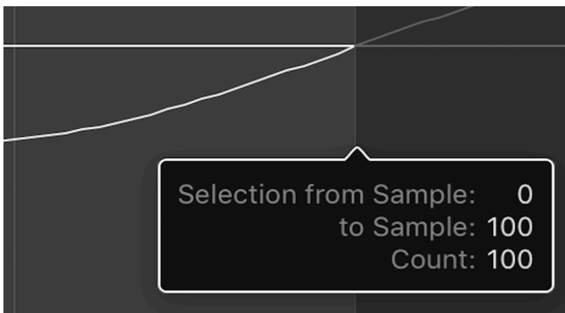
Figure 13c: detail from 441 Hz Sine wave bounced then confirmed as 100 samples in wave editor.
