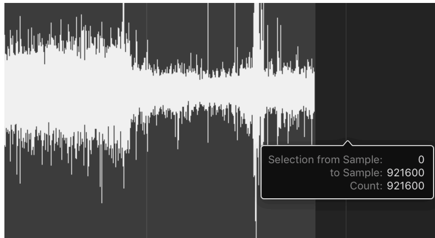
Figure 16: Conversion Image 2: Practical confirmation of length in samples from 256Hz to 44.1kHz conversion
