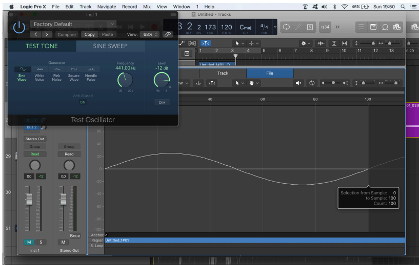
Figure 13a: 100 samples = 441 Hz confirmation via signal generator and bounced into wave editor.
