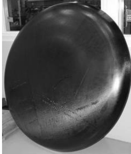
Fig. 10: Injected and cured dome shaped part
