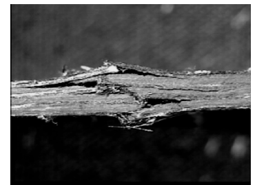
Fig. 4.35: H/W drilled RFI UCS failure
