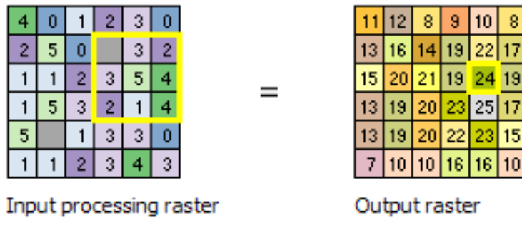
figure 4.2 Schematic for the application of focal statistics for raster (DTM) cell (ESRI, 2022).
